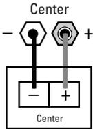
Speakers and electronics have corresponding (+) and (-) terminals. It is important to connect both speakers identically: (+) on the speaker to (+) on the amplifier and (-) on the speaker to (-) on the amplifier. Wiring "out of phase" results in thin sound, weak bass and poor imaging.
