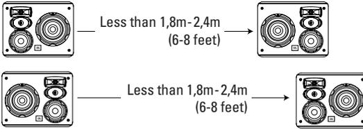
A wider stereo image is presented with the tweeter/midrange array outboard, and a tighter image is presented with the array inboard.
