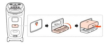
1. Pull down the latch to open the battery compartment, and then remove the old battery.
