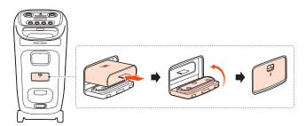
2. Insert a new battery of the same type (JBL BATTERY400) with the metal contacts facing down, and then close the battery cover.
