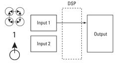
Selecting "1.2" in the input mixer sends a summed mono signal to the output. This selection is useful for sending a stereo signal to the mono output when using subwoofers intended to receive information from both the left and right inputs. (See Figure 2.)
