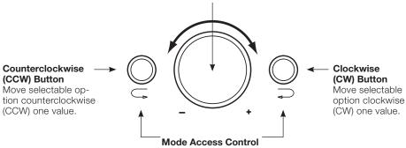
Pressing both the left and right buttons simultaneously for specified time periods accesses various modes of the amplifier.
