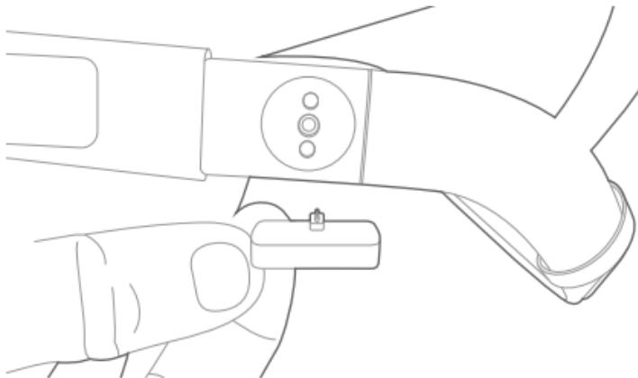
2. Place the head of the audio arm into the screw and hold it in place.
