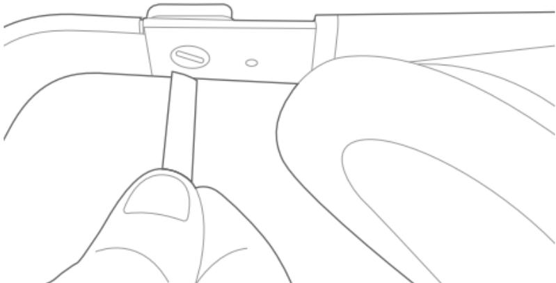
4. Turn the audio tool clockwise (to the right) to tighten the screw until it is secure.
