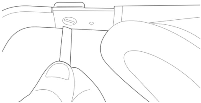
2. Turn the audio tool counter clockwise (to the left) to loosen the screw.
