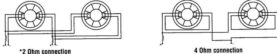
**\*Note:** We recommend both inputs of the woofer be driven by two separate channels of amplification (i.e. left channel of stereo amp to left terminals of the woofer and right channel of stereo amp to the right terminals). Do not connect just one set of woofer terminals as this alters the performance of the woofer.
