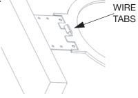
**Step 4:** After the wallboard is installed, cut out the hole for the speaker using the inside cutout of the frame as a guide. The speaker wire can then be run through the opening in the wallboard and attached to the speaker system – refer to the Owner's Manual of the loudspeaker for more information on system setup.
