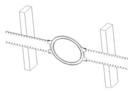
**Step 2:** Position the Rough-In Bracket/Wing assembly between the wall studs so that the bracket is in the correct position for the final speaker placement. Nail the assembly into place, making sure that the nail heads are as flush against the wings as possible.
