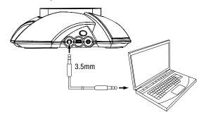
IMPORTANT: If you play audio through a docked iPod/iPhone and an audio source connected to the Audio In connection at the same time, you will hear *both* of their outputs mixed through the JBL On Stage Micro III. To hear only one source you will need to manually turn off the source you do not want to hear.
