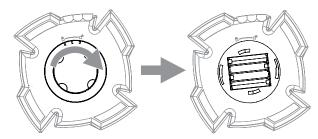
3. Insert four AAA batteries in the compartment. Observe the battery polarity that is indicated inside the battery compartment.
