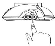
10. Adjust the volume using the (+) and (-) buttons. Press both buttons to mute the sound; press either button to unmute the sound.
