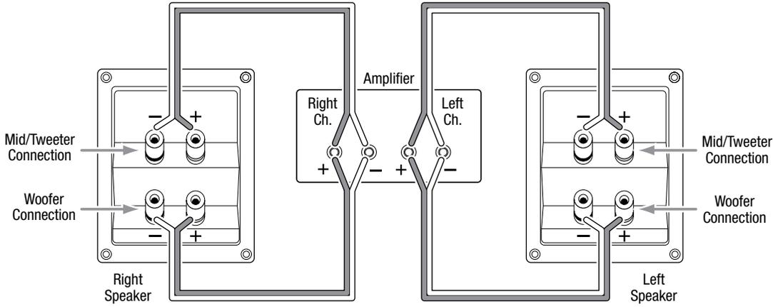
If you're bi-wiring with two stereo power amplifiers, connect the speakers according to the following illustration.
