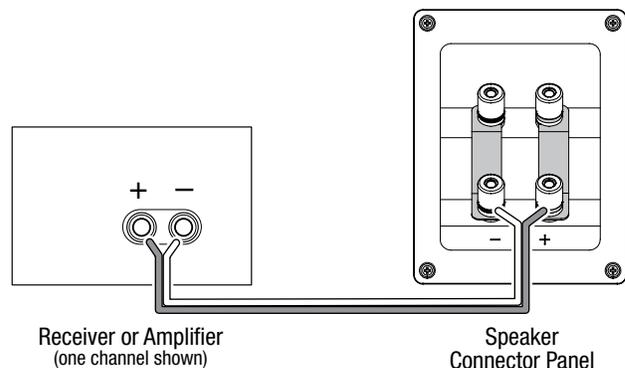
Connect the amplifier to each speaker as shown in the illustration on the right. You can use either set of terminals on the speaker. NOTE: Do not remove the metal jumpers from between the two sets of terminals when connecting the speaker wires.
