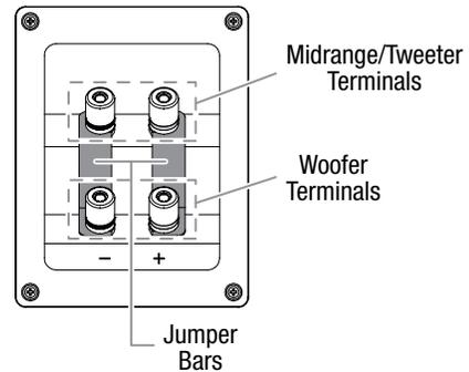
To bi-wire the 4319, first remove the terminal jumpers as shown in the illustration on the right.
