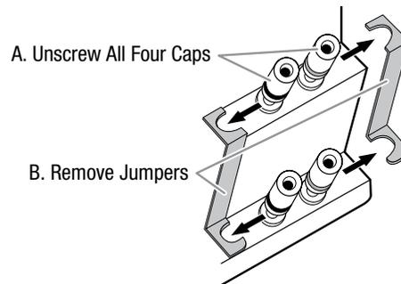
If you're bi-wiring with a single stereo power amplifier, connect the speakers according to the following illustration.
