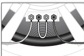
$$R_t = R_1 + R_2 + R_3 \dots$$
