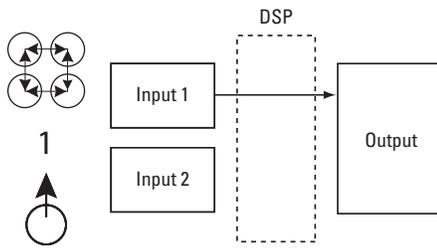
Selecting “1.2” in the input mixer sends a summed mono signal to the output. This selection is useful for sending a stereo signal to the mono output when using subwoofers intended to receive information from both the left and right inputs. (See Figure 2.)
