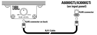
**Figure 1**. Connecting the Remote Level Control.
