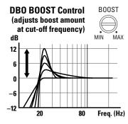
Figure 13. Frequency response curves show typical DBO control ranges for the JBL A6000GTi or A3000GTi amplifier.
