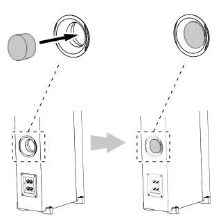
NOTE: The Studio 590 has two port tubes and includes two port tube inserts.
