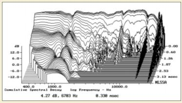
Fig.7 JBL S38, cumulative spectral-decay plot at 50" (0.15ms risetime).
