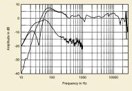
Fig.3 JBL S38, anechoic response on tweeter axis at 50", averaged across 30° horizontal window and corrected for microphone response, with the nearfield woofer and port responses and their complex sum plotted below 300Hz, 1kHz, and 300Hz, respectively.
