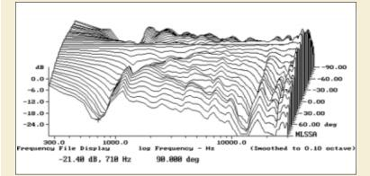
Fig.4 JBL S38, lateral response family at 50", normalized to response on tweeter axis, from back to front: differences in response 90°–5° off-axis on tweeter side of baffle, reference response, differences in response 5°–90° off-axis on woofer side of baffle.
