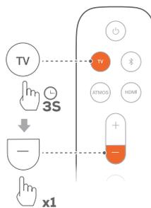
2. Within five seconds, press **+** or **-** on the remote control to switch between bass levels.
