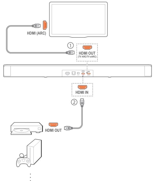
1. Make sure that the soundbar has been properly connected to your TV and digital device (See "5.1 Connection with your TV and digital devices" in the "5. CONNECT" chapter).
