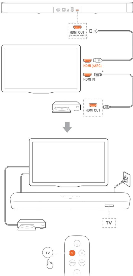
1. Connect the soundbar with the **HDMI IN (eARC)** connector on your TV by using the supplied HDMI cable.
