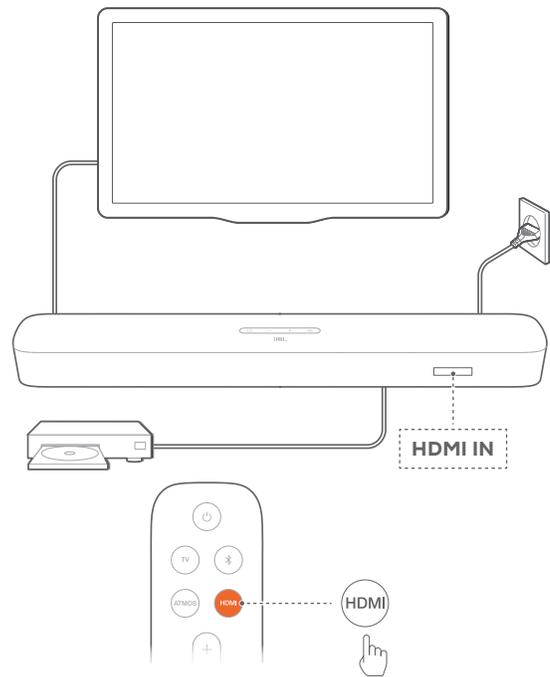
1. Connect the soundbar with the HDMI IN (ARC) connector on your TV by using the supplied HDMI cable.
