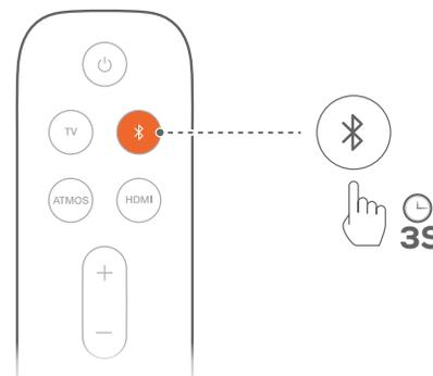
1. In the Bluetooth source, press and hold  $\text{G}$  on the soundbar or  $\text{B}$  on the remote control until “BT PAIRING” is displayed.
